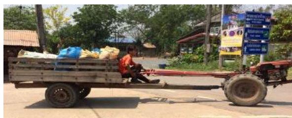
Photo 5. The modified pushing tractor attached on the wheel cart used in farming
