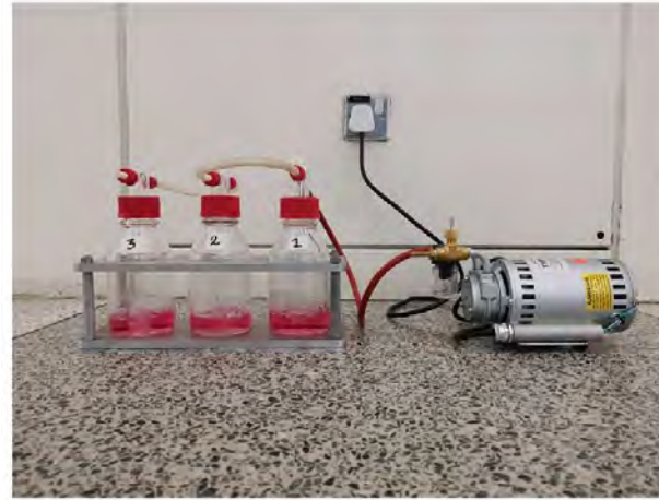
FIG. 17.1 The novel aerosol sampling setup. The three gas wash bottles filled with 100 mL of Trizol.
