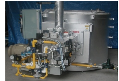
Regenerative Burners in industries, Toyotsu Machinery, Indonesia
