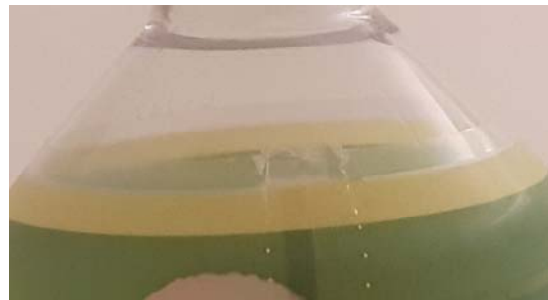
Perforation on the labeling of PET bottle.
