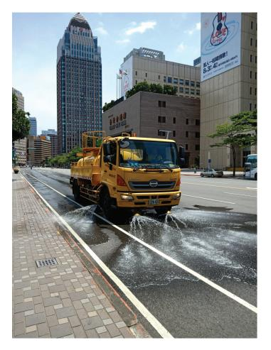
Sprinkling water to lower the surface temperature of roads in response to high temperatures
