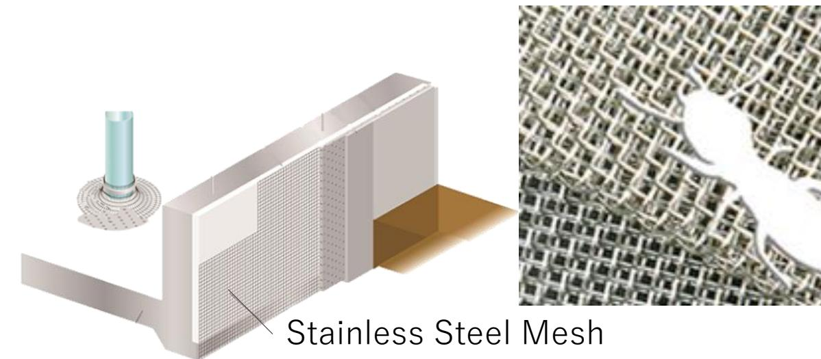
**A mesh smaller than the size of a termite head physically blocks termite invasion.**
