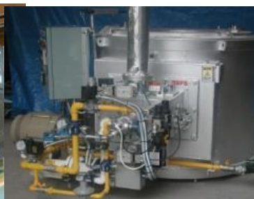
Regenerative Burners in industries, Toyotsu Machinery Indonesia
