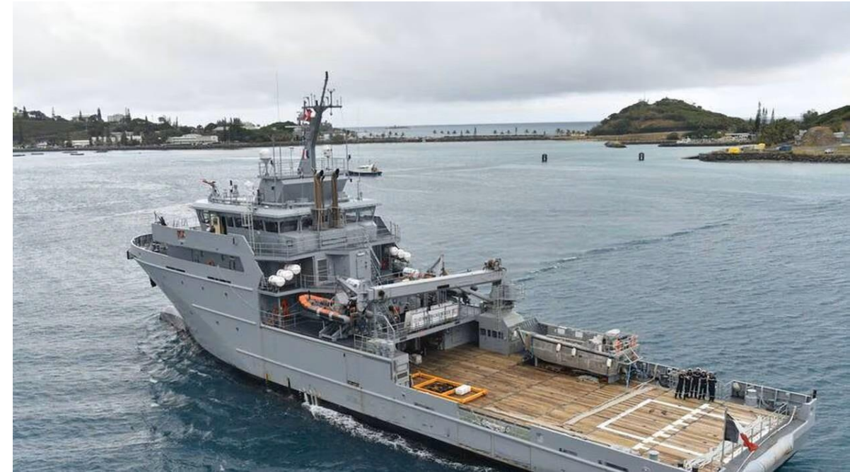
BSAOM: multi-purpose ship – large deck and containing capacity to support HDAR and depollution operations
