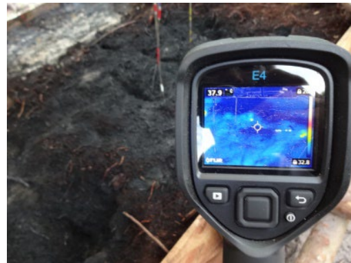
Firefighting using the backpack water tank with the portable infrared thermal imaging camera against hot spots over 50°C.
