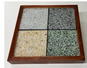
Concrete tiles made from T-eConcrete®/Carbon-Recycle
