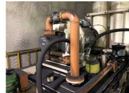
Pump: PV2R4 Motor: 45kW-6P
