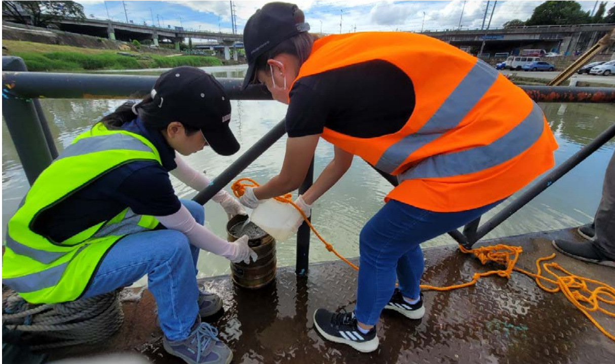
Figure 11. Collected surface water passes through a stack of sieves with decreasing mesh sizes from top to bottom
