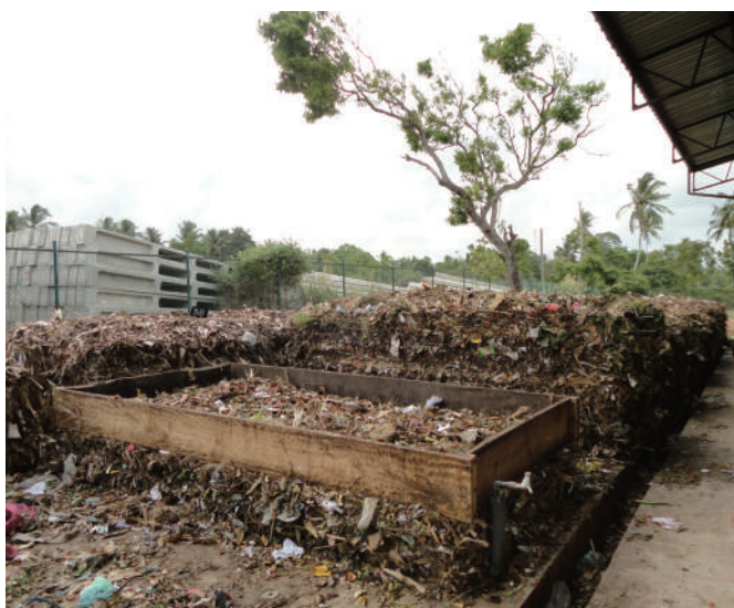
Figure 2-6 Piling up composting feedstock using wooden frame and skid steer loader (Source: author)
