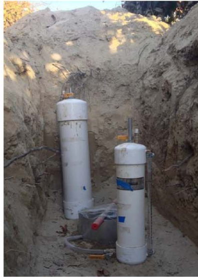
Figure 1 Infiltration Test with a Dual-ring Infiltrometer and Mariotte Bottles. Pre- and post-nitrate concentrations were measured and plugged into HYDRUS 1D model to assess immobile zone nitrate capturing potential.
