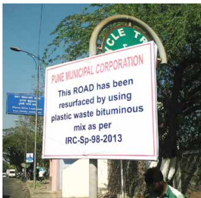
Figure 37: Road resurfaced using plastic waste bituminous mix
