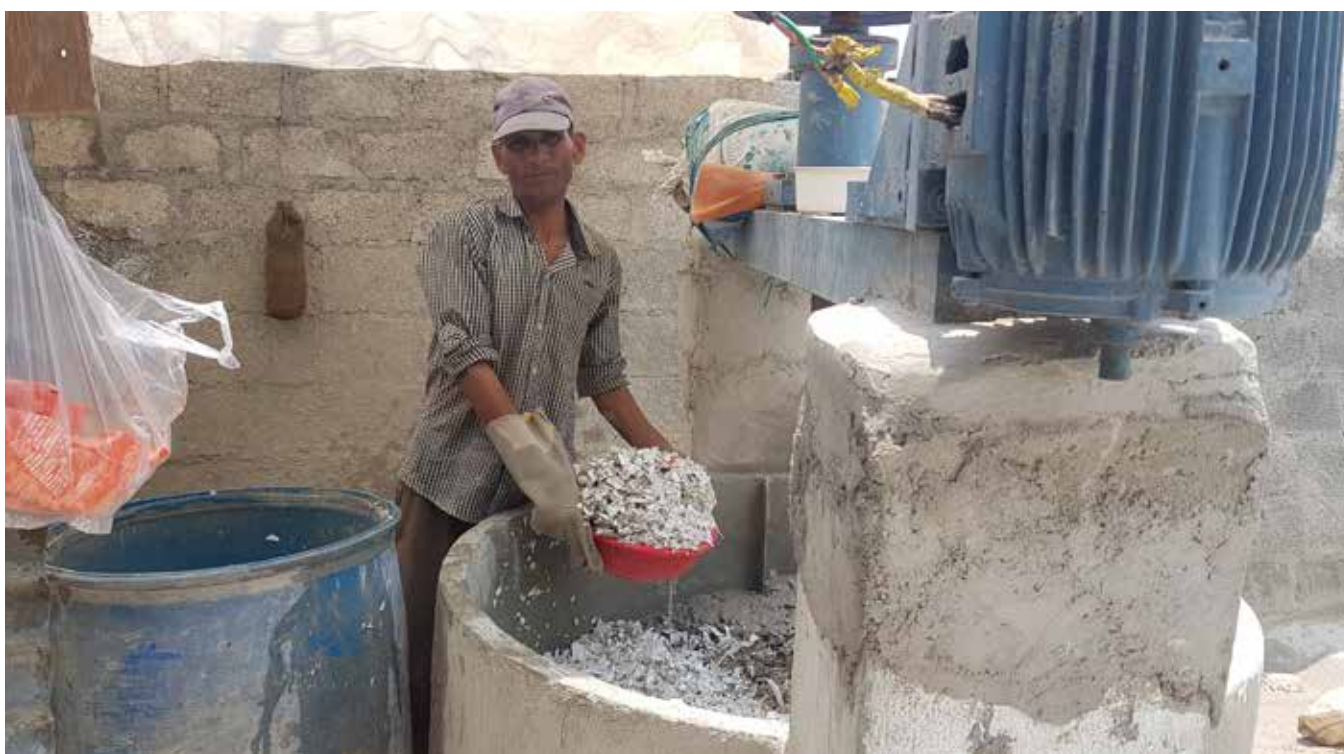
Figure 14: Semi-automated washing of shredded plastic
