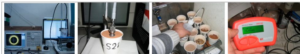
Figure 3. Dielectric constant measurement of soils in the laboratory using the dielectric probe toolkit.
