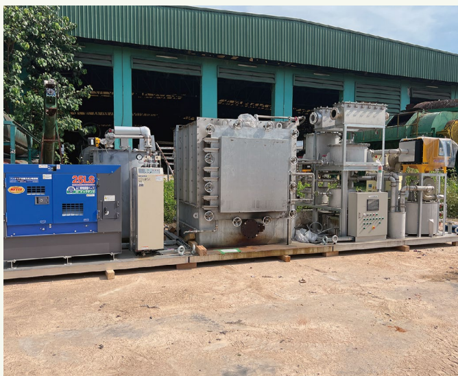
△ Waste plastic oil conversion system used in proof-of-concept tests
