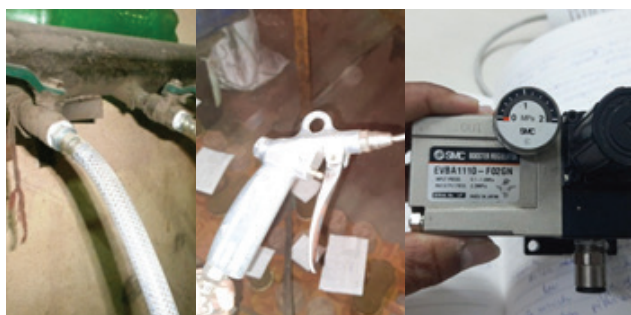
Figure 7. Optimizing compressed air system: (L-R): arresting leakages; use of air guns; monitoring air pressure
