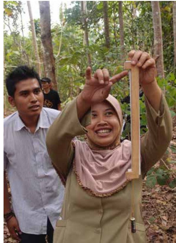
Picture 6. Using the Christen hypsometer
