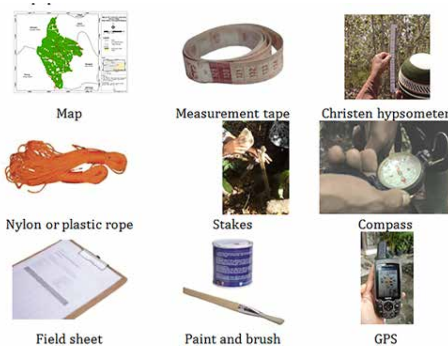
Figure 1. Tools and equipment for forest carbon accounting
