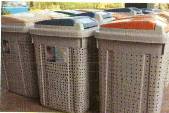
Aeration holes were made on plastic containers which were distributed to each household for composting.
