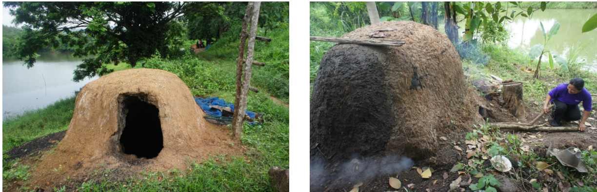
Figure 1 Charcoal production from eucalyptus wood residues using the earthen kilns
