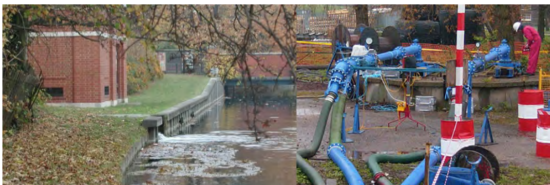
Figure 3. Test pumping an old, large diameter well in 2000 at 20,000 m 3 /d, and a modern NLARS borehole building with discharge into the New River. © Thames Water Utilities Ltd
