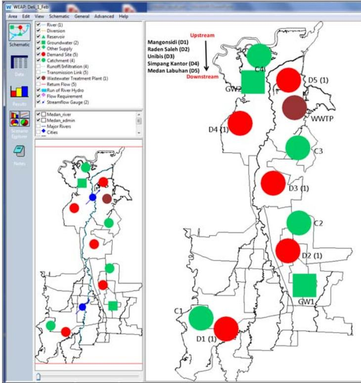
FIGURE 43.8 Schematic diagram showing the problem domain for water quality modeling in Medan using WEAP interface. WEAP, Water Evaluation and Planning.
