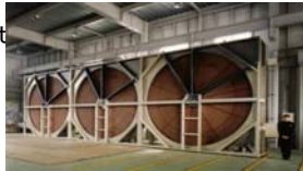
RTO (Regenerative Thermal Oxidizer), 1 set 蓄热燃烧装置1台
