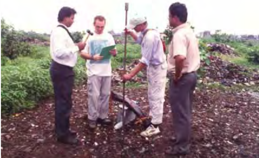
Methane Gas Emission is being measured by the expert of the Royal Haskoning of the Netherlands and Waste Concern by land fill gas analyzer at the Matuail Waste Disposal site of Dhaka City Corporation
